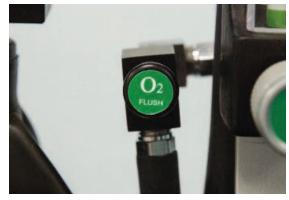
Do not use the flush valve when a patient is attached to the anesthesia machine.
