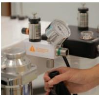
Attach a 1-liter reservoir bag to the limb under the Bain control arm.
