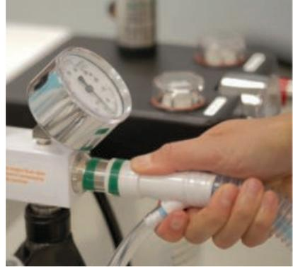
Connect the **exhalation tube** of the Bain circuit to the **exhalation tube** on the Bain control arm.
