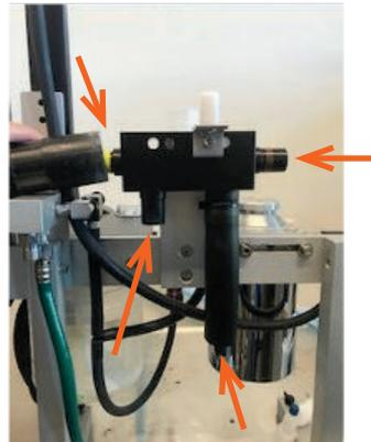
3 Replace tubing and 3L bag (if present) in accordance with the Anesthesia Breathing Circuit Standardized Color-Coding.
