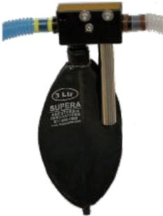
Ensure that a Y-adapter is in place and that the blue, corrugated scavenger tube is connected **FROM** the **scavenging limbs** on the Bain control arm to the cart's **outflow manifold**
