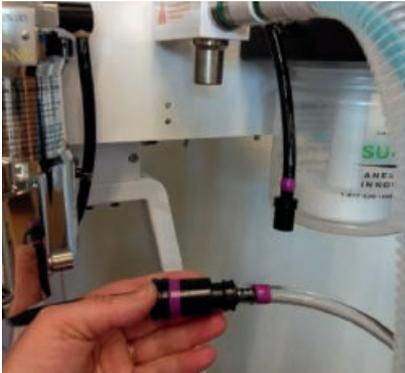
Connect the **clear, smooth inhalation tube** of the Bain circuit to the **fresh gas out-flow tube** on the anesthesia cart..
